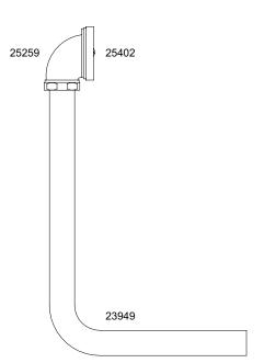
Chrome plated brass 1 1/4" x 14" x 18" Overflow tube 1 1/4" Satin chome plated elbow Stainless steel overflow strainer & screw
