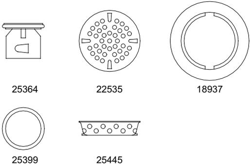
Handles and strainer are stainless steel. Drain body and stopper are nickel plated brass.
